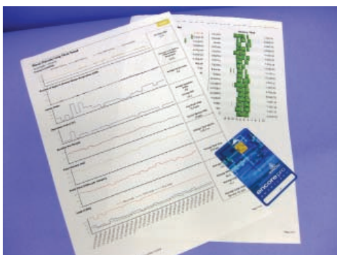
Figure 4 Smart cards and data download from home ventilators can provide clinically useful information regarding the effectiveness of ventilatory support over a prolonged time period. This information usually includes compliance, leaks, tidal volume or minute ventilation and machine settings.
