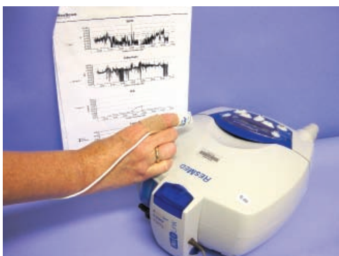
Figure 5 The addition of oximetry recordings to the download of machine performance can assist with clinical decision making regarding the effectiveness of current settings, the impact of events (e.g. leak) and the presence of persisting abnormal sleep breathing events.
